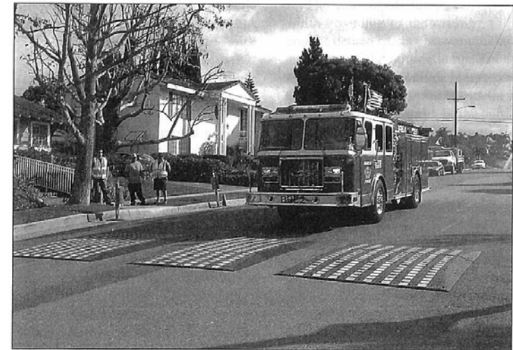
Figure 3. Testing City of Brea fire engine on speed lumps in La Habra, California.
